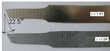
Figure 3; Failure along a plane inclined at a 22.5 degree angle to the maximum normal stress plane.
